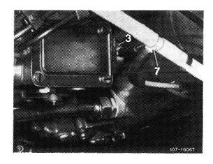
Unscrew pipe connection (1) of first injection pump element, removing compression spring (3) and delivery valve (4).
